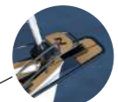
Easy removable stainless steel bowsprit for tacking of sails, anchor support and fitting a bow ladder.
