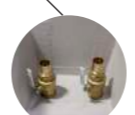
All through hull fittings are over dimensioned and fitted on single laminate. The reinforced hoses have twin clips in acid resistant stainless steel.
